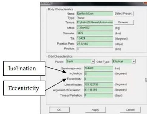
Figure 6. Changeable parameters in “Edit body” option in Astronomicon.
